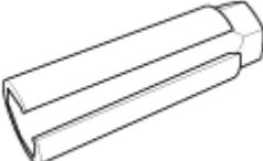
A long, tapered wrench with a hexagonal socket at the end, used for removing and installing heated oxygen sensors.                   | Removal and installation of the heated oxygen sensor<br>※ SST No.09392-2H100 model also can be used for removing the Heated Oxygen Sensor.                    |
