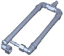
A U-shaped adapter with two fittings, designed to connect between a high pressure fuel pump and a low pressure fuel feed tube.        | Used for connecting between high pressure fuel pump and low pressure fuel feed tube to measure the pressure in fuel line<br>※SST 09353-C1000 also can be used |
